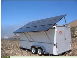
Electricity for various needs can be generated onsite by mobile systems that capture renewable energy.
