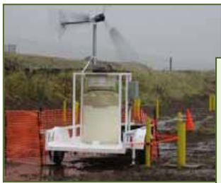
Recovery of petroleum products from groundwater at the former Adak Naval Complex in Alaska was powered by a mobile wind turbine.
